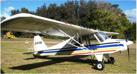
Bob's Karatoo J6 took just 18 months to complete. Bob is using a Honda Viking 100hp engine which is fitted with fuel injection and twin electronic ignition.
